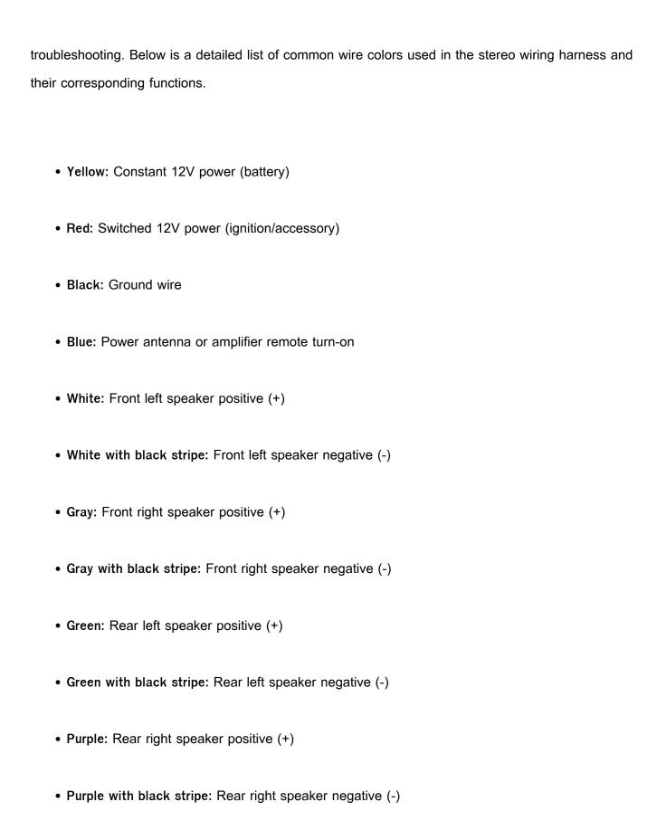
Understanding these colors ensures that the stereo receives power correctly, and audio signals are routed properly to each speaker. Miswiring any of these can result in no sound, distorted audio, or
