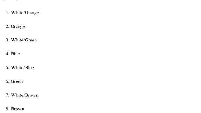
Trim the wires to a uniform length of about 1/2 inch to ensure they fit neatly into the IDC slots.
